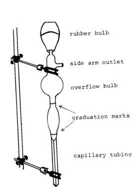
The viscometer was filled by compressing the bulb, covering the side arm, then slowly releasing the bulb. The upper clamp is then raised so the tip stays above the surface of the liquid. The flow was timed at the etched marks.
